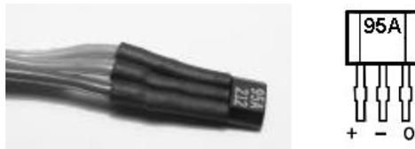
Now solder the other ends into the PC board in the same order as the component leads. Note that the part number and beveled faces are facing you as in the picture.
