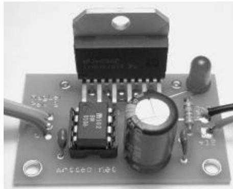
You can bolt the heat sink on at this time if you wish, the fins should face away from the board. All that remains is to solder 2 more wires at least 6” long into the holes on each side of U4. These wires will connect to your coil.
