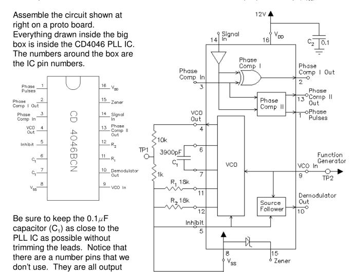
The data sheet for the CD4046 indicates that with  $R_1$  = 18k $\Omega$ ,  $R_2$  = 18k $\Omega$ ,  $C_1$  = 3900pF and  $V_S$  = 12V the VCO frequency range will be from 30kHz to 50kHz.
