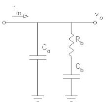
Note that the input of the loop filter is a current, rather than a voltage. That means that the output of the phase detector must be converted from a voltage to a current. The voltage to current circuit that we will use is called a *charge pump*. The whole phase-locked-loop circuit is shown below, including the charge pump and the filter from the previous page as the loop filter.
