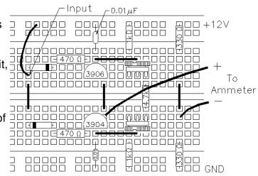
connections for current measurements) and/or fuse. If the ammeter is working but you can't obtain the correct reading, check the top diode and the 2N3906 for proper installation.
