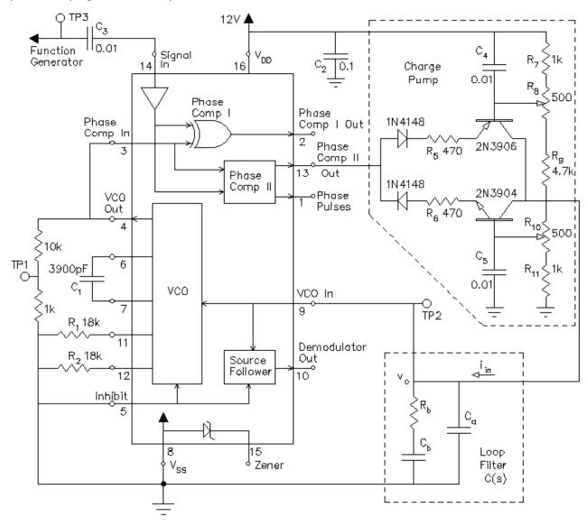
Assume that the "plant" transfer function is  $P(s) = \frac{kpll}{s}$  With  $k_{pll} = 2.435 \frac{Amp}{Volt \sec}$
