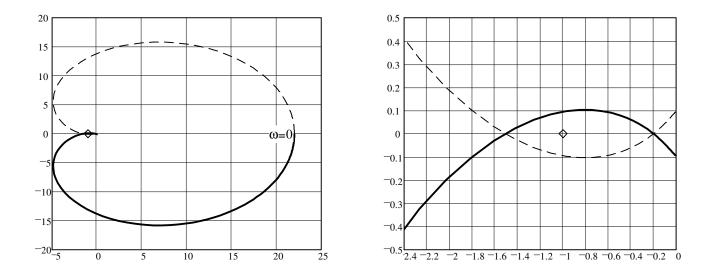
b) Repeat part (a) for the system whose Nyquist curve is shown at below (or in text), given that the system has one unstable pole.
