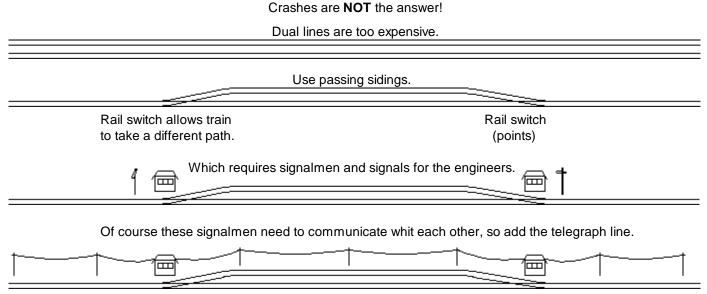
Clearly this is a system which cries out for a more automated approach, but remember, this is before computers, before logic gates, before transistors, even before vacuum tubes. I know, it's hard to imagine, but such times *did* exist.
