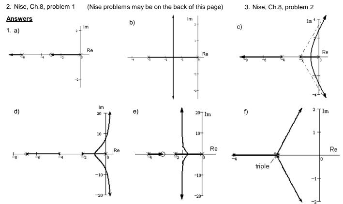
2. a) No: Not symmetric; On real axis to left of an even number of poles and zeros
