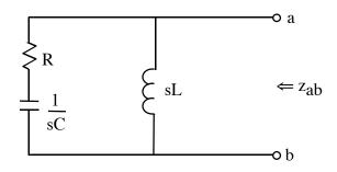
$$z_{ab} = \frac{s\left(Rs + \frac{1}{c}\right)}{\frac{R}{L}s + \frac{1}{LC} + s^{2}} = \frac{Rs(s + 1/RC)}{s^{2} + \frac{R}{L}s + \frac{1}{LC}}$$
