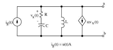
Construct an s-domain Thevenin's equivalent to the circuit at the terminals a-b. There is no initial energy stored in the circuit.
