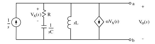
$V_{Th}(s) = V_0(s)$  with no load across a, b terminals.
