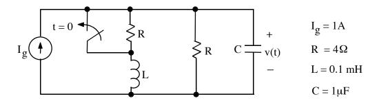
The current source is a dc current source. After being open for a long time, the switch is closed at t = 0.
