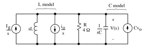
**Note:** A DC source corresponds to a step function <u>even if there is no switch and the source has the same output for all time.</u> Thus, we have  $I_g/s$  as the source in the *s*-domain. (Conceptually, we only need the current source for t > 0 because the initial conditions on L and C account for what the current source did for t < 0.)
