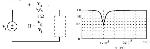
Using not more than one each R, L, and C, design a circuit to go in the dashed-line box that will produce the |H| vs.  $\omega$  shown above, that is:
