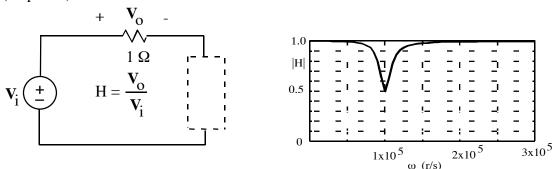
Using not more than one each R, L, and C, design a circuit to go in the dashed-line box that will produce the |H| vs.  $\omega$  shown above, that is:
