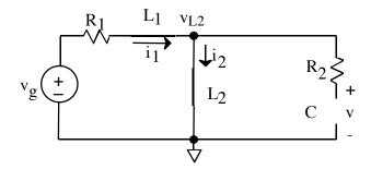
Since no current flows through  $R_2$ , we may find  $i_1$  (which equals  $i_2$ ) from the loop on the left side.
