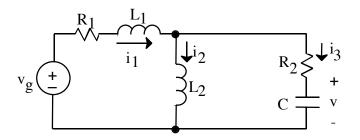
At t = 0,  $v_g(t)$  switches instantaneously from  $-v_o$  to  $+v_o$ .
