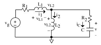
We treat  $L_1$  and  $L_2$  as current sources and v as a voltage source, and we solve for  $v_{L1}$ ,  $v_{L2}$ , and  $i_C$  using standard techniques (such as node-voltage or superposition). Each variable we are solving for is the voltage for a current source or the current for a voltage source. Thus, they are variables we solve for indirectly: we solve the circuit and then use Kirchhoff's laws to find the value we are looking for in terms of other values.
