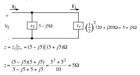
sol'n: (b) Our first step is to convert our circuit to a Y - Y form so we can use a single-phase equivalent model. In this problem, the circuit is already in Y - Y form and we may draw the single-phase equivalent directly:
