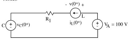
We may apply any standard method to solve the circuit, but we can solve the above circuit using a voltage loop.
