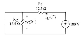
$$i_L(0^-) = \frac{100\text{V}}{25\Omega} = 4\text{A}$$
