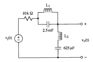
Find values of L<sub>1</sub> and L<sub>2</sub> for the above filter circuit such that the transfer function equals zero for the sixth harmonic and zero for the twelfth harmonic of periodic  $v_i(t)$  that has period  $T = 2\pi/60$  s.
