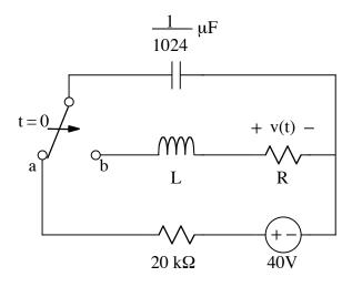
In the above circuit, the switch moves from a to b at t = 0.
