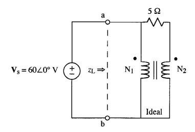
Given  $N_1/N_2 = 9$ , calculate the impedance,  $z_L$ , seen by the voltage source in the above transformer circuit.
