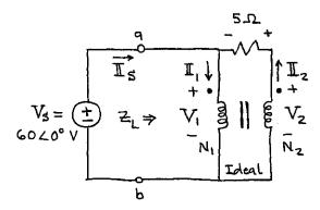
Note: The + signs for  $V_1$  and  $V_2$  are at the dots. I, flows into the dot, and II, flows out of the dot.
