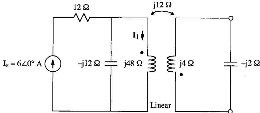
Calculate the numerical value of phasor current  $I_1$ .
