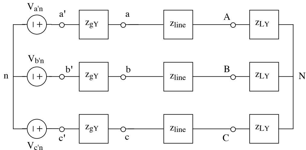
$$\begin{array}{ll} V_{a'n} = 82\angle 0^\circ \text{ V} & z_{gY} = 0.1 \Omega \\ V_{b'n} = 82\angle 120^\circ \text{ V} & z_{line} = 39 + j5 \Omega \\ V_{c'n} = 82\angle -120^\circ \text{ V} & z_{LY} = 0.9 + j4 \Omega \end{array}$$
