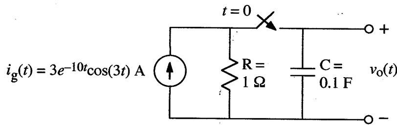
**Note:** The initial voltage on the capacitor is  $v_C(t = 0^-) = 3 \text{ V}$  measured with + on top.
