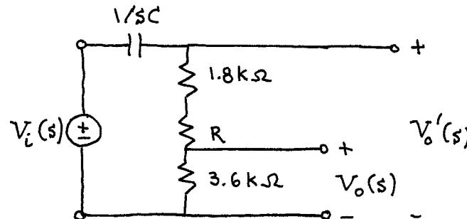
In this configuration we have a standard RC filter multiplied by a voltage divider.
