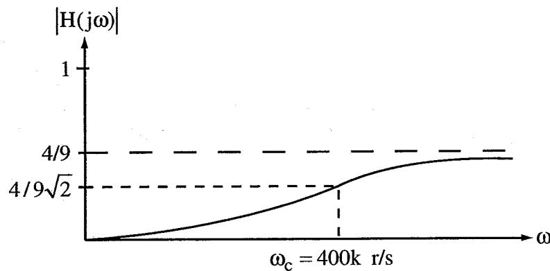
Using not more than one each R, L, and C, design a circuit to go in the dashed-line box that will produce the  $|H(j\omega)|$  vs.  $\omega$  shown above, that is:
