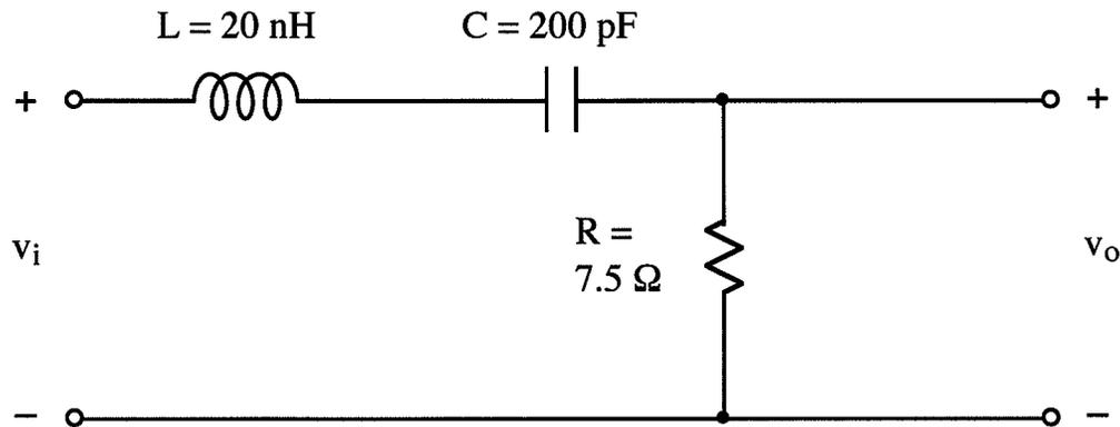
For the band-pass filter shown above, calculate the following quantities:
