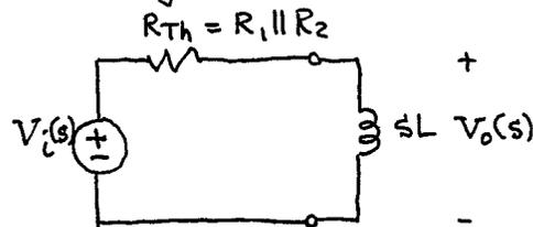
For this filter, we have  $H'(s) = \frac{sL}{sL + R_{Th}} = \frac{1}{1 + \frac{R_{Th}}{sL}}$ .
