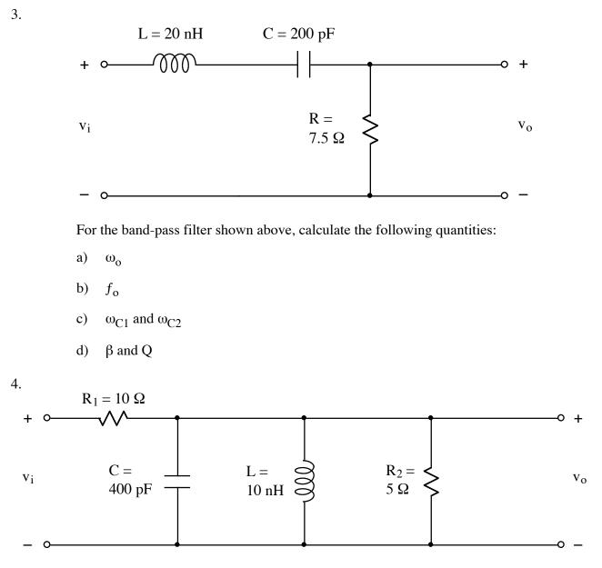
For the band-pass filter shown above, calculate the following quantities: **Hint:** Use a Thevenin equivalent for the R's.
