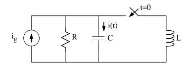
After being open for a long time, the switch closes at t = 0. The inductor carries no current at time  $t = 0^-$ . Give expressions for the following in terms of  $i_g$ , R, L, and C:
