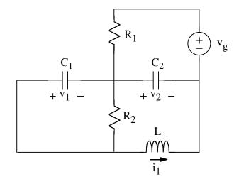
At t = 0,  $v_g(t)$  switches instantly from  $-v_o$  to  $v_o$ .
