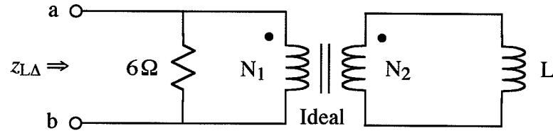
Given  $N_1/N_2 = 2$  and  $\omega = 100 \text{ rad/s}$ , find a numerical value for  $L$  to make  $z_{L\Delta} = 3 + j3 \Omega$ .
