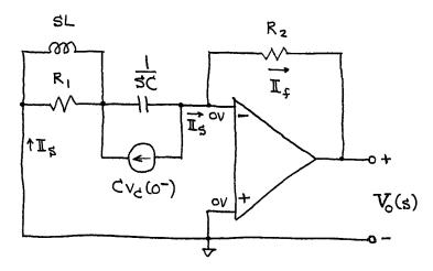
To solve this op-amp circuit, we observe that  $V_+ = OV$  and  $V_- = V_+ = OV$ .
