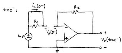
The op-amp has negative feedback that acts to keep  $V_- \doteq V_+$ . Thus, we have OV at the inputs of the op-amp.
