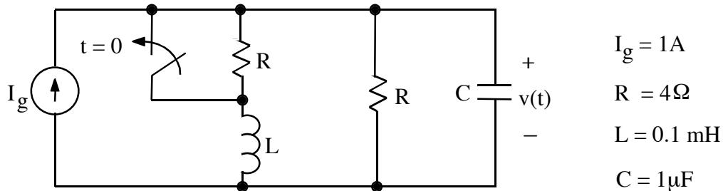
The current source is a dc current source. After being open for a long time, the switch is closed at  $t = 0$ .
