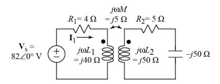
Calculate the numerical value of phasor current,  $I_1$ , flowing into the primary side of the transformer. Note: the transformer is linear.
