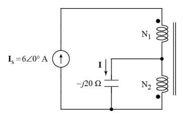
The turns ratio of the transformer is  $N_1/N_2 = 6$ . Calculate the numerical value of phasor current, **I**, flowing down through the capacitor. Note: the transformer is ideal.
