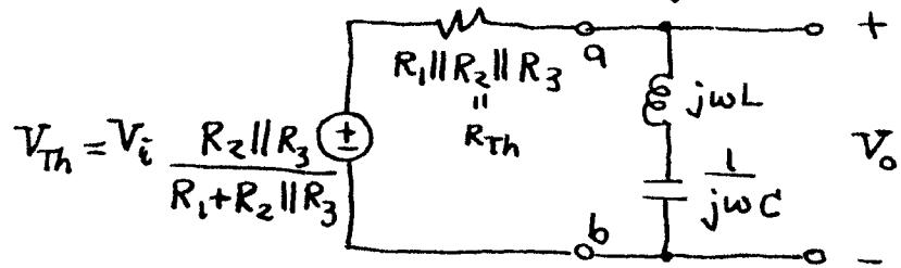
$$\text{Note: } \frac{R_2 \parallel R_3}{R_1 + R_2 \parallel R_3} = \frac{R_1 \parallel R_2 \parallel R_3}{R_1} = \frac{R_{Th}}{R_1}$$
