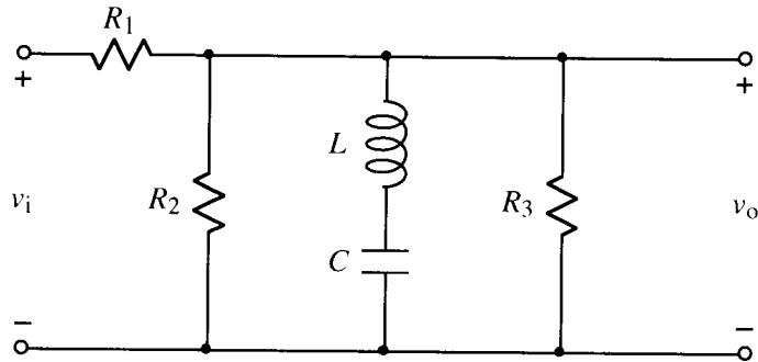
$$R_1 = 18 \Omega \quad R_2 = 48 \Omega \quad R_3 = 144 \Omega \quad C = 31.25 \mu\text{F} \quad L = 2 \text{ mH}$$
