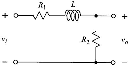
$$R_1 = 150 \Omega \quad R_2 = 750 \Omega \quad L = 1 \mu\text{H}$$
