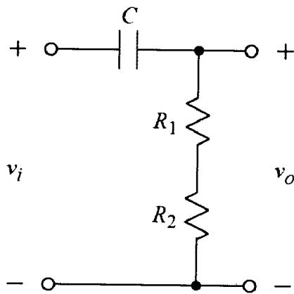
$$R_1 = 120 \text{ k}\Omega \quad R_2 = 130 \text{ k}\Omega \quad C = 200 \text{ nF}$$
