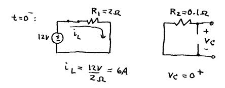
At t=0+, we can model the L and C as sources, since  $i_L(0^+)=i_L(0^-)$ ,  $v_C(0^+)=v_C(0^-)$ , and any component whose i or v is known may be replaced by a source with that i or v value.
