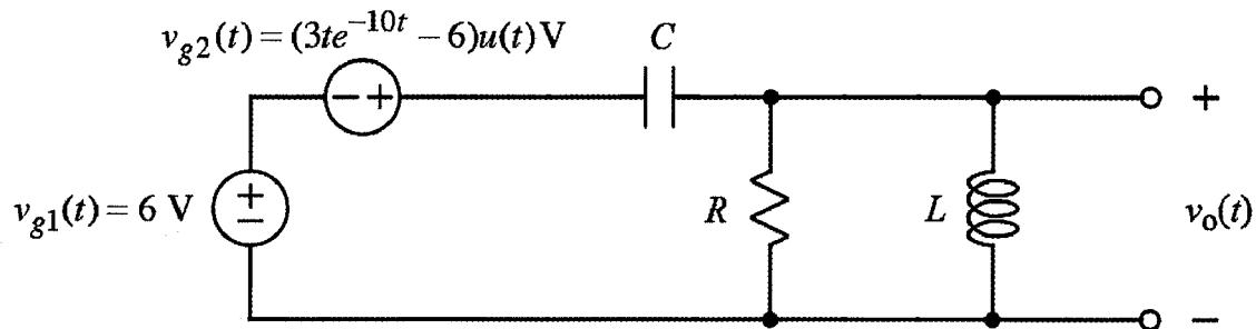
Note: The 6 V in the  $v_{g1}(t)$  source is always on.
