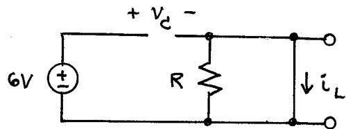
Using an outside  $v$ -loop, we find that we must have  $v_C = 6V$ .
