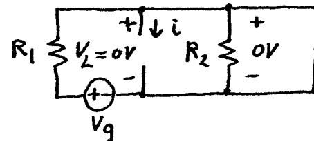
The wire (the  $C$  with  $0V$ ) bypasses  $R_2$ .
