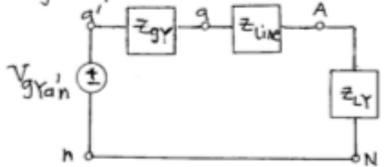
$$V_{gY_a/n} = 71.0 \angle -30^\circ \text{ V}$$
