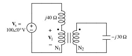
Given  $V_1 = 150 \angle 0^{\circ} V$  find the turns ratio,  $N_1/N_2$ , for the transformer in the above circuit. Note: the transformer is ideal.
