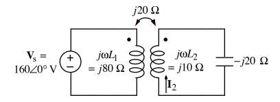
Calculate the numerical value of phasor current,  $I_2$ , flowing upward in the right coil of the transformer in the above circuit. Note: the transformer is linear.
