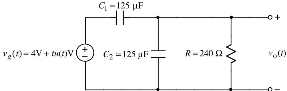
**Note:** The 4 V in the  $v_g(t)$  source is always on.
