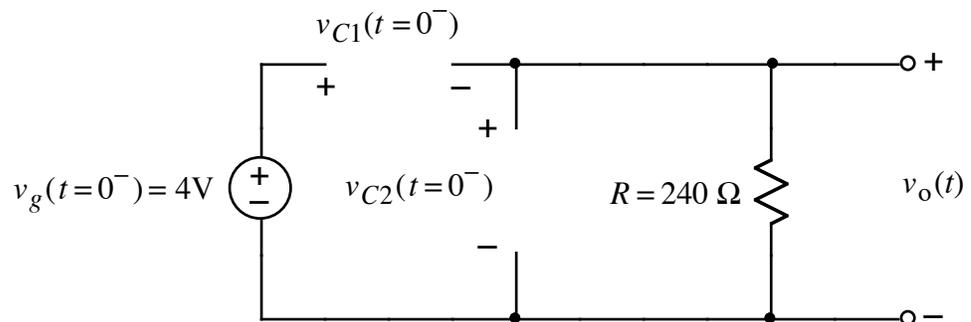
The  $R$  discharges  $C_2$  so all of the source voltage appears across  $C_1$ :
