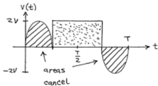
We spread the remaining rectangle across one period, resulting in a height of  $1V$ .
