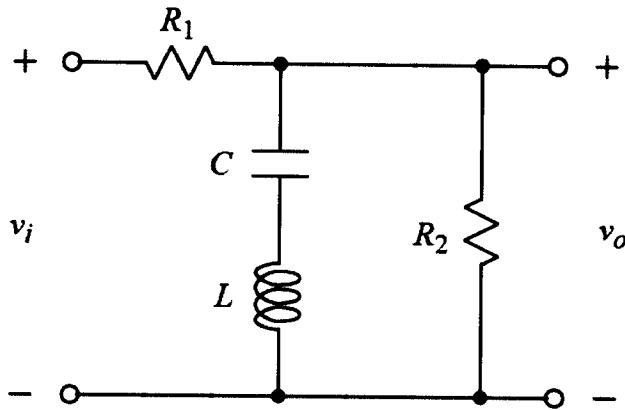
$$R_1 = 18 \Omega \quad R_2 = 36 \Omega \quad C = 31.25 \mu\text{F} \quad L = 2 \text{ mH}$$
