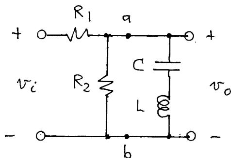
We remove  $L$  and  $C$  to find the Thevenin equivalent of  $v_i$ ,  $R_1$ , and  $R_2$ . We then measure the voltage across  $R_2$ . The voltage-divider formula yields the answer:
