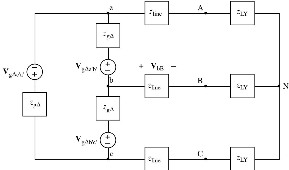
$$V_{g\Delta a'b'} = 168 \angle 0^\circ \text{ V} \quad z_{g\Delta} = j0.9 \Omega$$
