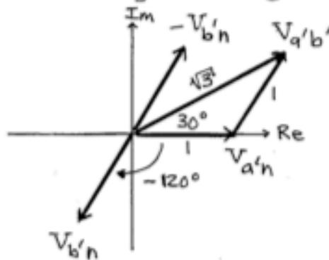
$$V_{q'b'} = V_{a'n} - V_{b'n} = V_{a'n} - V_{a'n} \cdot 1 \angle -120^\circ$$
