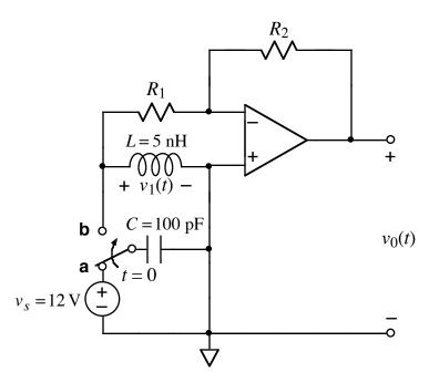
After being in position **a** for a long time, the switch moves to position **b** at time t = 0.
