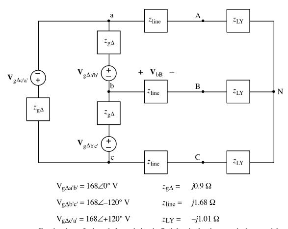
For the above 3-phase balanced circuit, find the single-phase equivalent model.
