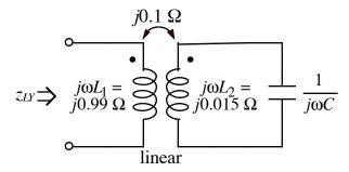
Given  $\omega = 1 \text{M rad/s}$ , find the value of C that makes  $z_{\text{LY}} = -j1.01 \,\Omega$ . Note that  $z_{\text{LY}}$  is the equivalent impedance of the entire circuit.
