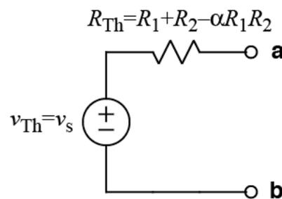
**NOTE:** An alternative approach is to use a current divider to find an equivalent resistance for the dependent source. The current through  $R_1$  splits into two parts, and we can equate the current in the dependent source with the current that would flow in an equivalent resistance,  $R_{eq}$ .
