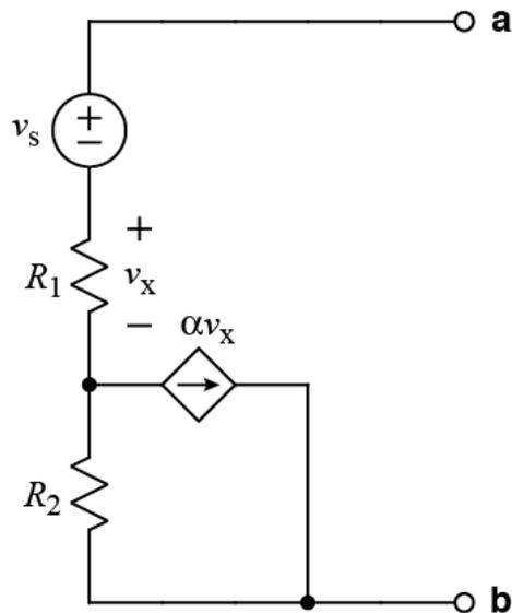
Find the Thevenin equivalent circuit at terminals **a** and **b**.  $v_x$  must not appear in your solution. **Note:**  $\alpha \neq 0$ .
