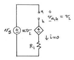
Because we have an open circuit i=0, and R has no v-drop. For a v-loop, we get
