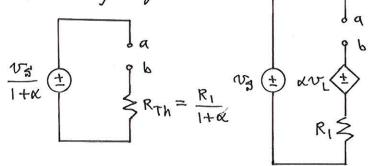
We could remove the  $\alpha v_L$  source and consider it to be part of the  $R_{Th}$ , if we also adjust the independent source. If we accept this change in  $v_s$ , then our  $\kappa v_L$  source becomes an  $R_{Eq}$ :
