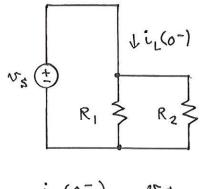
$$i_L(o^-) = \frac{v_S}{R_1 \parallel R_2}$$
