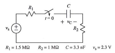
After being open for a long time, the switch closes at t = 0. The initial voltage on the capacitor is  $v_C(t = 0^+) = 1.5 \text{ V}$ . Hint: think Thevenin equivalent for the circuit the capacitor is connected to.
