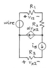
Because  $R_3$  is in series with  $i_{\sharp}$ , we use Ohm's law to calculate  $v_{\chi 2}$ .
