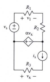
Using superposition, derive an expression for  $v_1$  that contains no circuit quantities other than  $i_s$ ,  $v_s$ ,  $R_1$ ,  $R_2$ ,  $R_3$ , and  $\alpha$ , where  $\alpha > 0$ .
