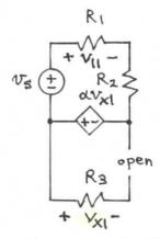
No current flows in R3, so  $V_{X1} = 0 V$ .
