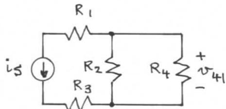
We may combine  $R_2$  and  $R_4$  into an equivalent resistance with  $v$ -drop  $v_{4I}$  across it. Then we have a resistance
