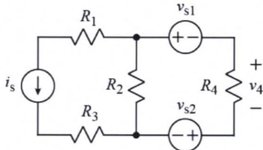
Using superposition, derive an expression for  $v_4$  that contains no circuit quantities other than  $i_s$ ,  $v_{s1}$ ,  $v_{s2}$ ,  $R_1$ ,  $R_2$ ,  $R_3$ , and  $R_4$ .
