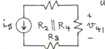
$$v_{4I} = -i_s \frac{R_2 R_4}{R_2 + R_4}$$
