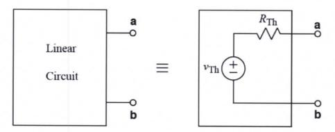
A linear circuit has a Thevenin equivalent, as shown above. Now suppose that components are added to that circuit as shown below.
