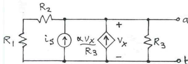
We have both the voltage and current for the dependent source as functions of  $V_x$ , allowing us to find an equivalent  $R$  value.
