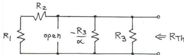
$$\text{So } R_{Th} = (R_1 + R_2) \parallel \frac{-R_3}{\alpha} \parallel R_3 \text{ as before.}$$
