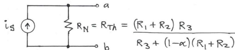
SOL'N: 3.a) The maximum power transfer occurs when the load resistance equals the Thevenin equivalent resistance, which may be shown by writing an expression for the power as follows and setting the derivative with respect to  $R_L$  equal to zero:
