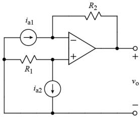
The op-amp operates in the linear mode. Using an appropriate model of the op-amp, derive an expression for  $v_0$  in terms of not more than  $i_{a1}$ ,  $i_{a2}$ ,  $R_1$ , and  $R_2$ .
